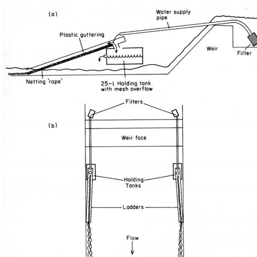
Figure 6.14. Pass-trap design from White and Knights (1994).
